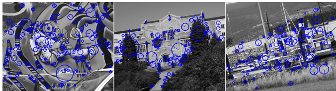
Fig. 4. Keypoint detection results for “graf”, “ubc”, and “boat” images. Each circle represents a keypoint, its radius indicating the scale of the feature. The lines in the circle represent orientation of the keypoints. Numbers of keypoints are 269, 133, and 192, respectively.
